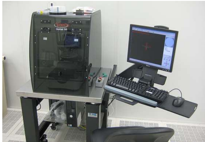
Figure 4.3 The device used for roughness determination
